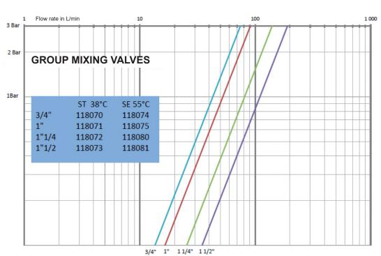
For optimal operation, it is recommended that your supply pressure is 3 bars and does not go beyond pressure drops of 1 bar.
