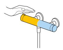
**touchcontrol** (on thermostats only) This water guidance system with its 'double skin' principle ensures that users are never burned by their KWC faucet. The insulated hot water supply keeps the body of the faucet warm without letting it get too hot.
