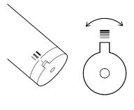
**smartcontrol** (on thermostats only) smartcontrol keeps an eye on water consumption. Tangible resistance in the turning handle limits the amount of outflowing water. To switch off the economy mode, twist the handle back past the catch point.
