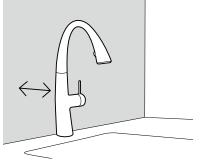
When installing faucets, the distance from the wall must be taken into account. Approximately 55 mm between the wall and the centre of the faucet.
